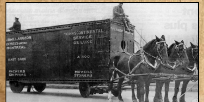
1907 - A fireproof, dual-control truck developed by the Montreal transportation company J.B. Baillargeon Express. A Teamsters driver is stationed at each end of the vehicle.
